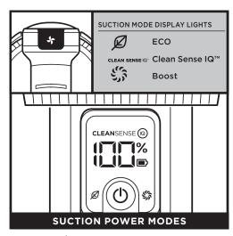
Press the (4) button to toggle between ECO, Clean Sense IQ™, and Boost modes. To save battery power, select ECO mode. For everyday cleaning power, select Clean Sense IQ mode. For an extra burst of power, select Boost mode.
