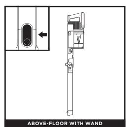
Stand the vacuum upright and press the nozzle release button located at the bottom of the wand. above the nozzle. Lift wand to detach.
