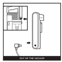
Press and hold the **Battery Release Button**, then slide out the battery. Plug the charger into the charging port on the battery. To reinstall the battery, slide it into the slot in the back of the handheld vacuum until it clicks into place.
