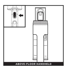
Press the wand release button and lift the handheld vacuum off the wand. An attachment can be used to clean stairs, furniture, and other above-floor areas.
