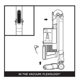
To put the vacuum in storage mode, press the Flexology Wand Unlock Latch while folding the handheld vacuum forward until the wand clicks and locks. Plug the charger into the charging port on the handheld vacuum.
