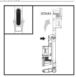
To take the vacuum out of storage mode, press the unlock latch and lift up the handheld vacuum until the wand clicks and locks into place.
