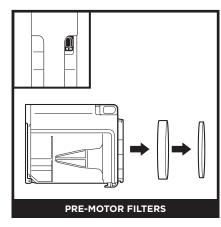
Remove the dust cup, and pull the foam and felt filters out of the back of the dust cup.
