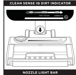
The **Clean Indicator** visually confirms when floors are cleaned. When the unit senses heavy debris, suction will increase for more cleaning performance. When the debris is cleared, suction will decrease. The clean indicator displays the level of debris detected. For best results, continue cleaning until the indicator returns to its lowest level before moving to the next area.
